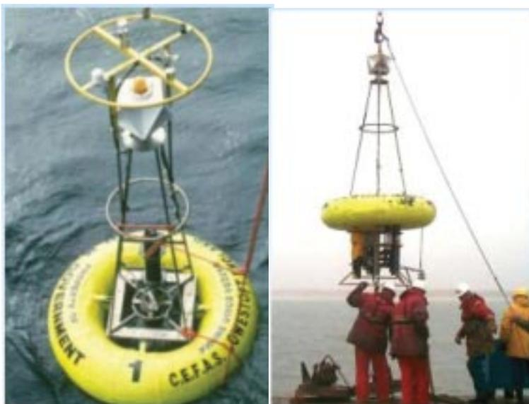
Figure 1 (above). CEFAS SMART Buoy recovery.
