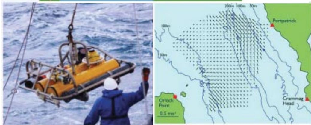
Fig. 3a (above left) ADCP recovery. Fig. 3b (above right) mean current in North Channel measured by HF radar.
