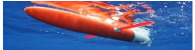
A spray glider, which is the platform used to collect the data visualized in the image to the left.
